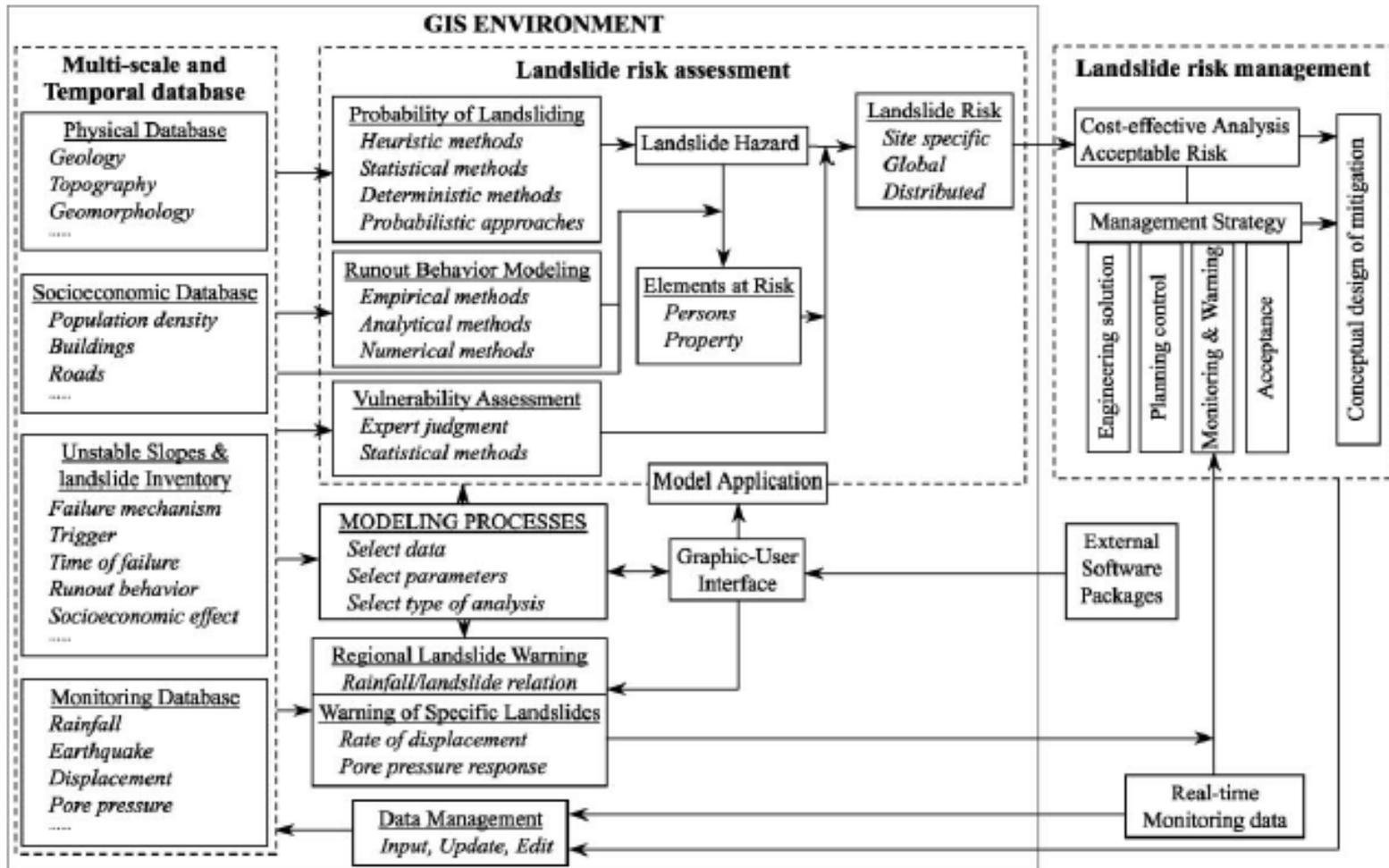
Proposed GIS-based conceptual integrated system for landslide risk assessment and management (Dai et al., *Eng. Geology*, 64, 65-87)
